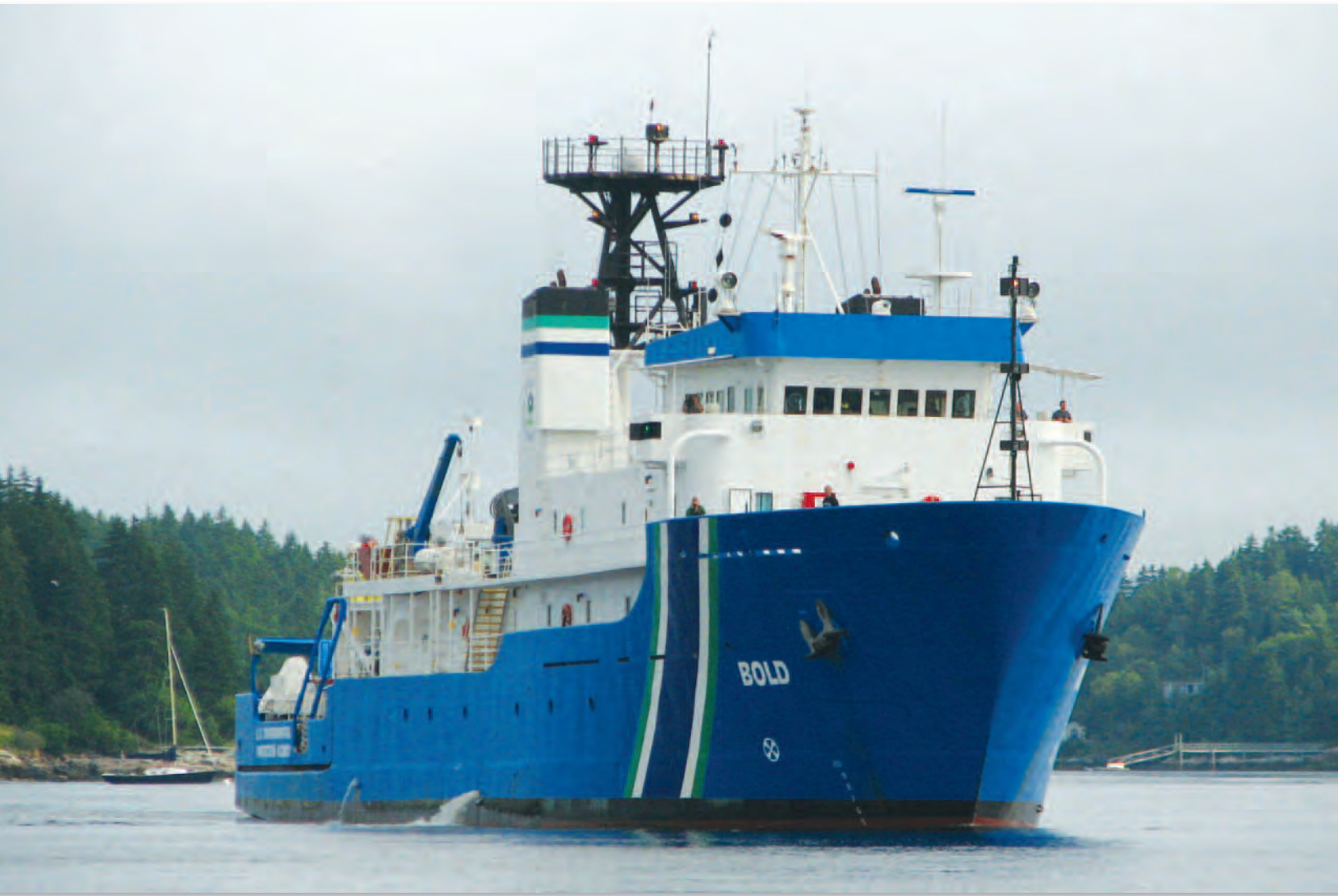
OSV Bold is the Environmental Protection Agency's only ocean and coastal monitoring ship. Bold, a converted MSC T-AGOS-class ship, is equipped with state-of-the-art equipment, including side-scan sonar, underwater video, water-sampling instruments and sediment-sampling devices. MSC contracted for the operation and maintenance of this ship on behalf of the EPA. U.S. Environmental Protection Agency photo by Cindy Falvey.
