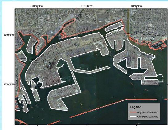
Fig 3. Example of varying coastline needs. Two coastlines were developed for the region surrounding the Los Angeles and Long Beach harbors. The red coastline does not include the large wharves resting on pilings and was used to build an intermediate model of seafloor relief. The white coastline, which includes the wharves, was used to clip the seafloor relief model and ensure that the wharves had positive elevation values in the final DEM.
