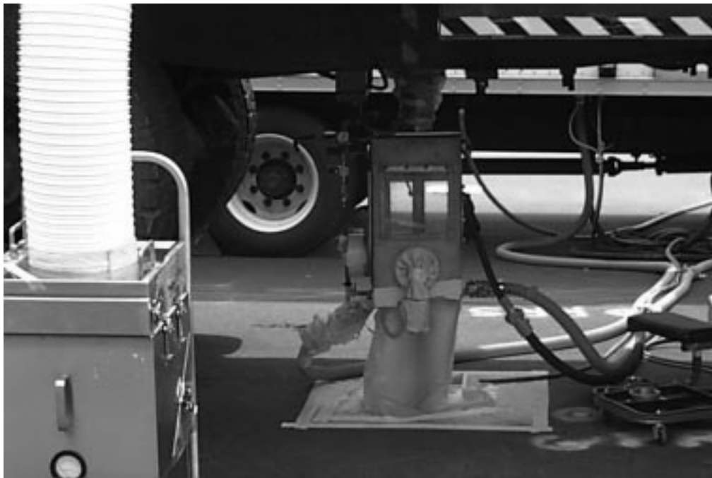
Figure 4. Glove box decontamination system designed for the SCAPS truck.
