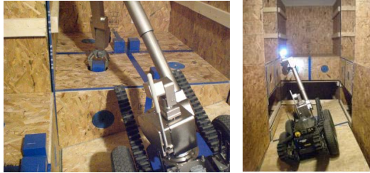
Directed Perception and Grasping Dexterity Test Method
