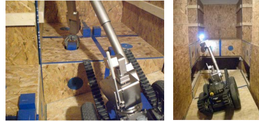
Directed Perception and Grasping Dexterity Test Method
