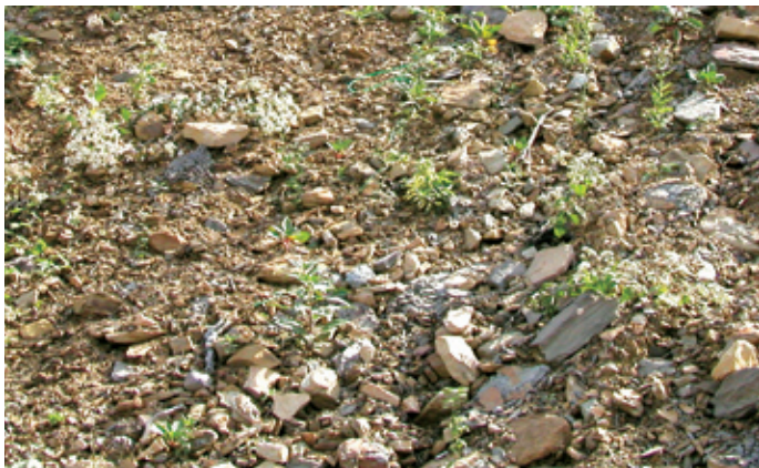
Photo 2. A mixture of brown weathered and gray sandstones, loosely graded to form a soil medium suitable for trees in West Virginia.
