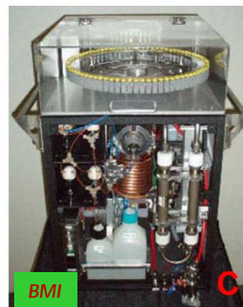
Figure 1 (A) –10 stage cascade Multi Orifice Uniform Deposition Impactor (MOUDI); (B) modified Davis Rotating drum Universal size-cut Monitoring impactor (DRUM); (C). Particle-to-Liquid Sampler (PILS).
