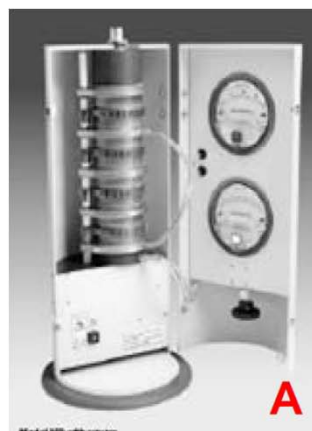
Figure 1 (A) –10 stage cascade Multi Orifice Uniform Deposition Impactor (MOUDI); (B) modified Davis Rotating drum Universal size-cut Monitoring impactor (DRUM); (C). Particle-to-Liquid Sampler (PILS).
