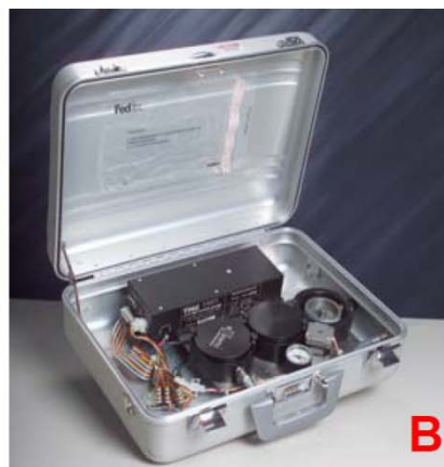
Figure 1 (A) –10 stage cascade Multi Orifice Uniform Deposition Impactor (MOUDI); (B) modified Davis Rotating drum Universal size-cut Monitoring impactor (DRUM); (C). Particle-to-Liquid Sampler (PILS).
