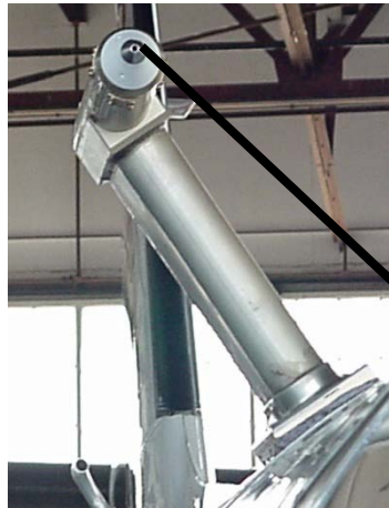
CVI inlet (aerosol from evaporated cloud particles when in clouds)
