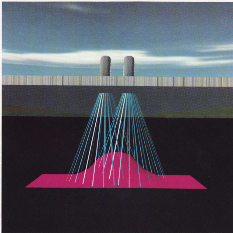
Figure 7b. Flexible Pavement with Multiple Wheel Load Showing Interaction
