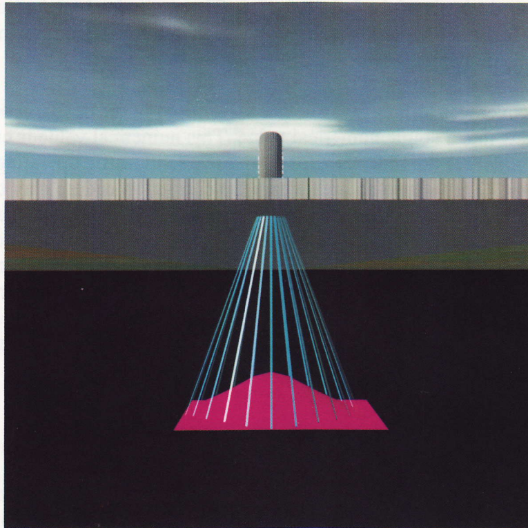
Figure 7a. Flexible Pavement with Single Wheel Load
