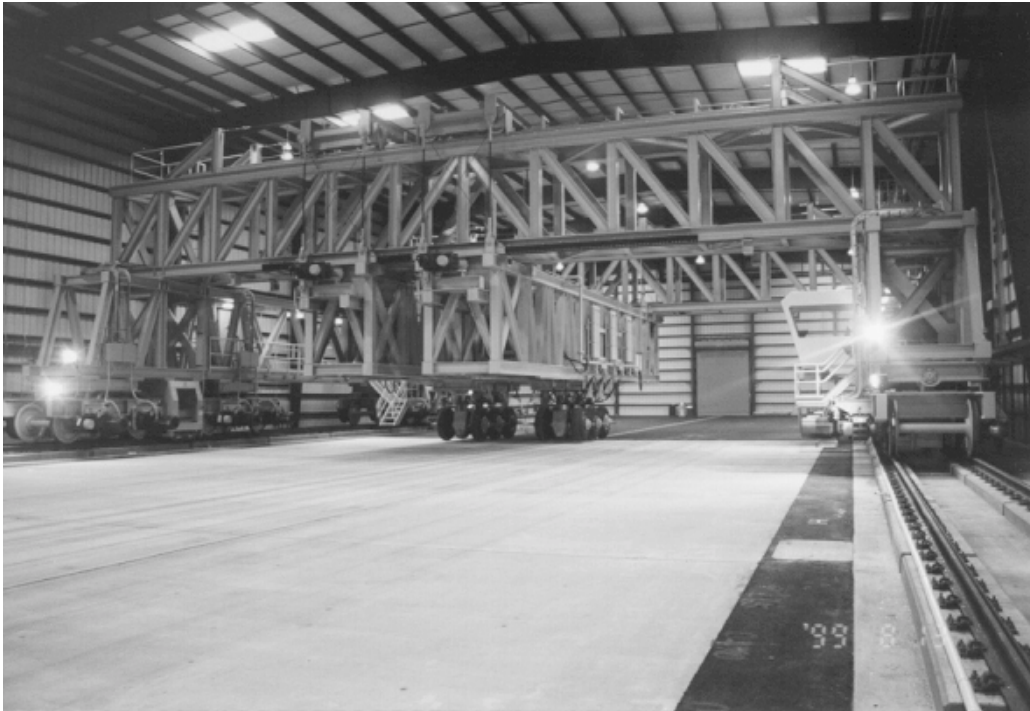
Figure 1. National airport pavement test facility (NAPTF). The test vehicle is shown at the start of LRS.
