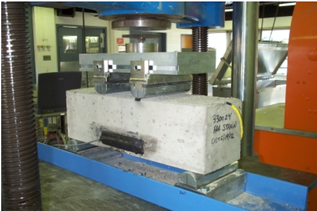
Figure 3 – Flexural Test of Beam
