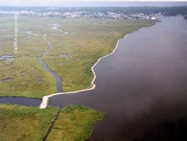
(L) Shoreline protection shields interior marshes from erosion and saltwater intrusion. (R) Shielding deteriorated landward marshes, the thin sliver of headland between Pass Chaland and Grand Bayou Pass provides a critical first line of defense against gulf storms.
