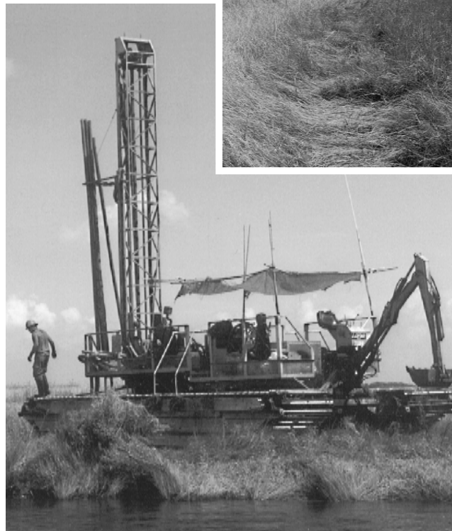
Aluminum marsh buggies, like the one shown above, do less damage to marsh areas than their steel predecessors.
