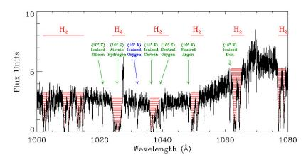
The data your satellite produces might look like this real data from the spectrograph on the Far Ultraviolet Spectroscopic Explorer (FUSE) satellite, which was launched in 1999. The ultraviolet spectrum above, which shows intensity of light over a range of wavelengths, is of a quasar called ESO141-G55.
