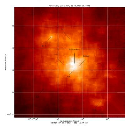
The data your satellite produces might look like this real data of the galaxy NGC 253 from the ASCA satellite, a Japanese X-ray astronomy mission launched in 1993. ASCA had two Solid-state Imaging Spectrometers (SIS), which were CCDs that could image as well as measure the position, time, and brightness of X-rays. From this information, graphs like light curves (intensity over time) and spectra (intensity over different wavelengths) can be made.
