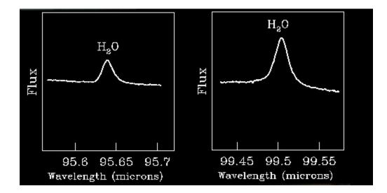
The data your satellite produces might look like this real data from the Infrared Space Observatory (ISO), a European satellite launched in 1995. ISO had four instruments, including a camera (ISOCAM), a photometer (ISOPHOT), and two spectrometers (SWS and LWS). These spectra, graphs of intensity of infrared light over different wavelengths (or energies), are from the Long Wave Spectrometer (LWS), and they show the presence of water vapor near the Orion Nebula, a star-forming region.
