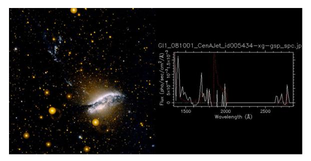
The data your satellite produces might look like this real data from the GALEX mission, which had a single instrument onboard that was both an imager and a spectrometer at UV wavelengths. Having just one instrument that can do multiple things is a good way to maximize science results on smaller missions where there may not be much money or space.
