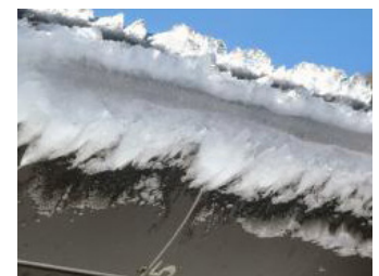
Ice accreted from super-cooled water droplets on the wing leading edge of a research aircraft while in cloud (Left) and after ascending above cloud (Right). Photo credits: NASA Glenn Research Center.
