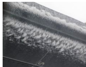
Ice accreted from super-cooled water droplets on the wing leading edge of a research aircraft while in cloud (Left) and after ascending above cloud (Right). Photo credits: NASA Glenn Research Center.
