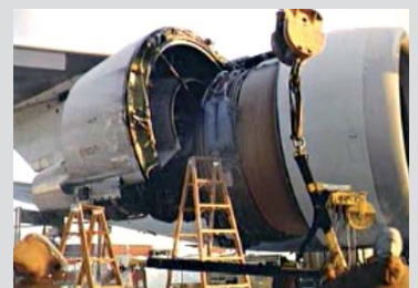
Image of the December 1989 Mt. Redoubt eruption (Upper) demonstrates that a large quantity of volcanic ash can be rapidly injected to aircraft cruising level. Heavy ash fall from this eruption also caused significant engine damage to a KLM passenger jet (Lower).
