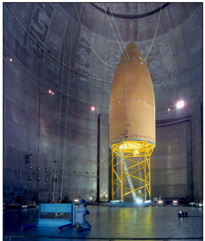
Ariane 5 payload fairing test in the SPF.
