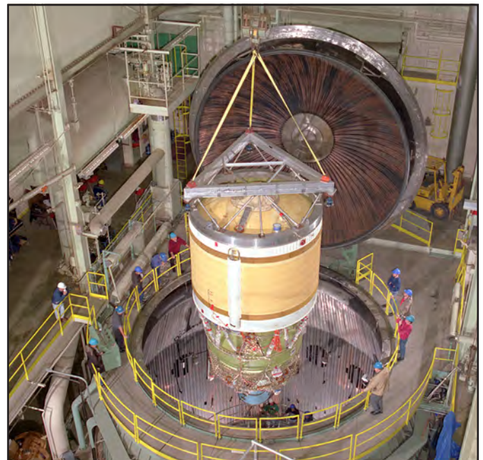
Boeing Delta III upper stage test at the B-2 test facility.
