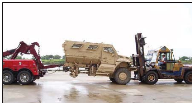
Battle-damaged Mine Resistant Ambush Protected vehicles AP's are discharged using "tandem" methods.
