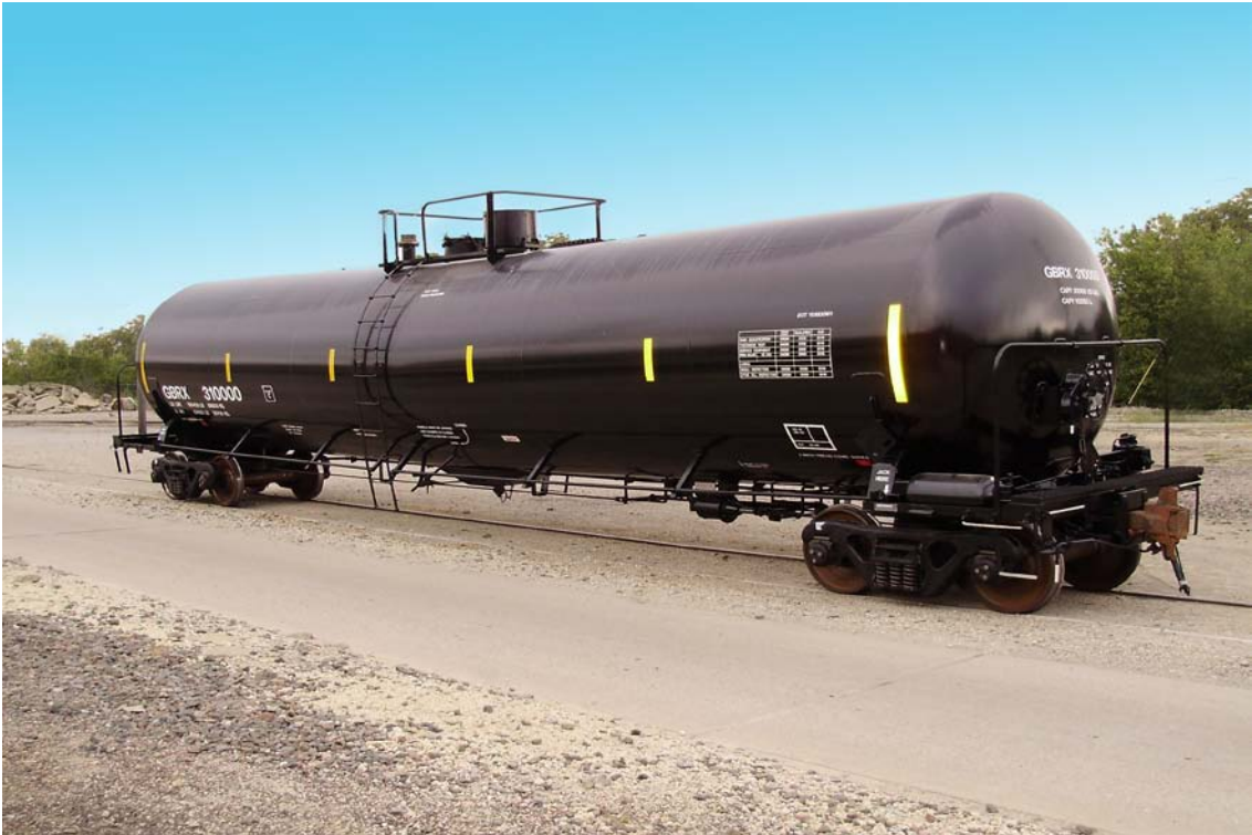
Tank car designed for the transportation of lubricating oil and similar fuel oil products.
