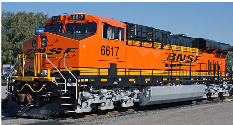
FIGURE 1 A typically configured diesel-electric locomotive
