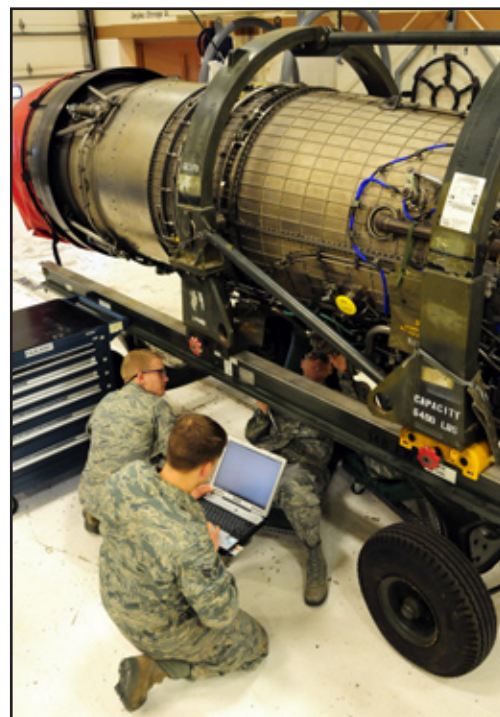
Airman 1st Class Matthew McEwen, Senior Airman John Broberg and Airman 1st Class Alicia Jenness conduct repairs on a dismantled F-16 Block 50 engine. Photo by Staff Sgt. Donald Acton.
