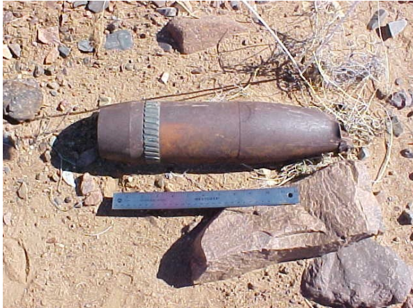
Photograph 5: Live 105mm Projectile, M314 Series with Fuze Found During USA's Investigation January 2004
