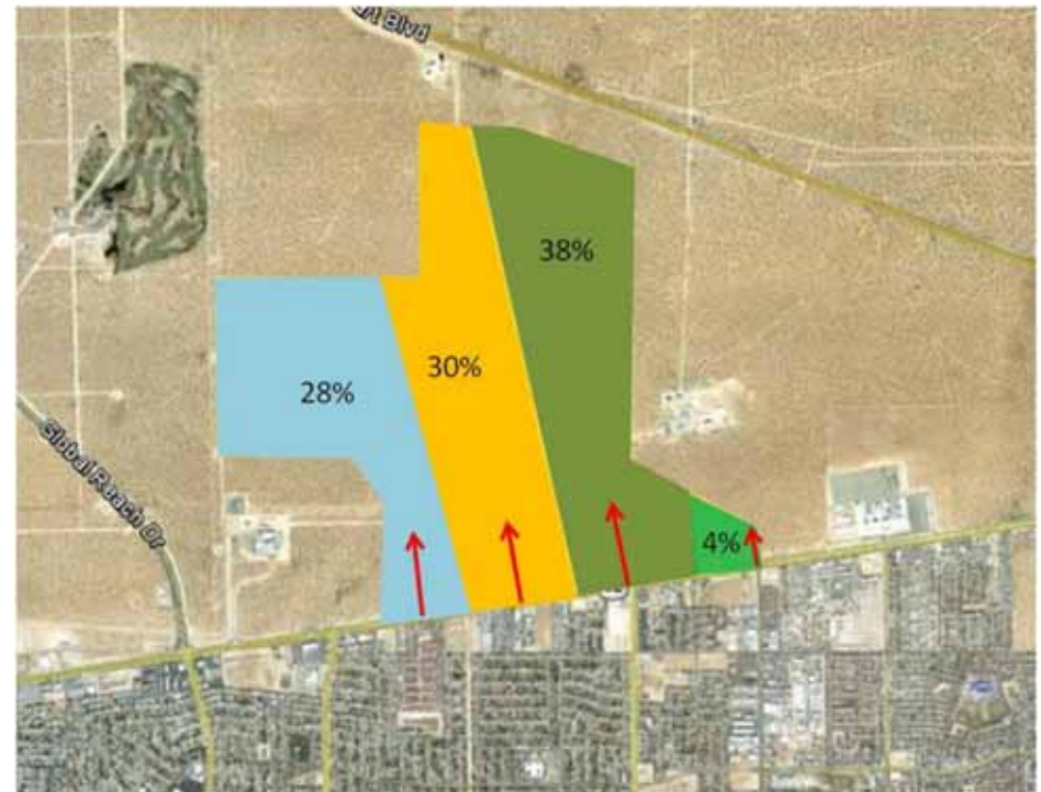
Fig. 62. George Dieter access traffic to parcel A is distributed by tributary areas
