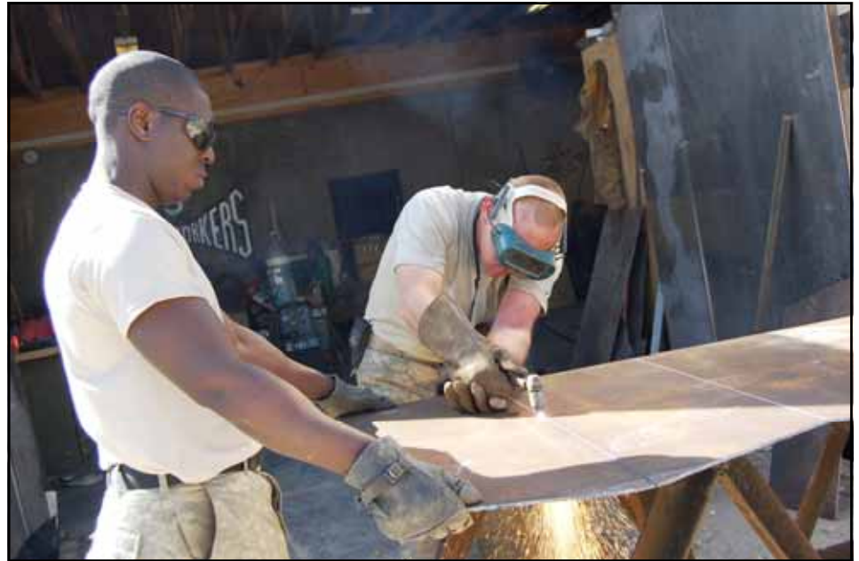
Spc. Leighton Jones, 24, of Fort Monroe, Virginia (left) holds a piece of steel in place as Sgt. Robert Smith, 39, of San Antonio, Texas (right) cuts it to the needed size to add to the turret of a vehicle March 31 at Forward Operating Base Orgun-E. Both Soldiers are assigned to Easy Company, 1 st Battalion, 503 rd Parachute Infantry Regiment.
