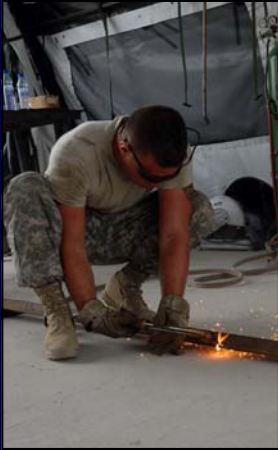
Pfc. Clayton Taylor, a metal worker with B Company, 173rd Brigade Support Battalion from Bamberg, Germany, cuts some angle iron to use it for a construction project in the B Company motor pool on Sept. 27, 2007.
