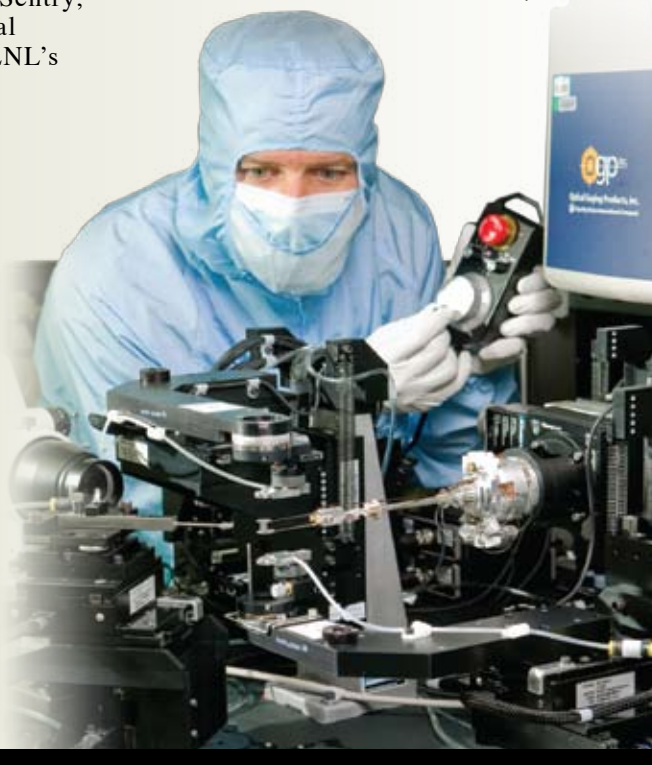
LLNL systems engineer Richard Montesanti operates the precision robotic assembly machine.
