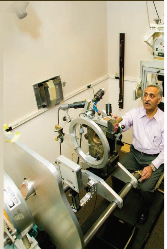
Inder Daftari, a medical physicist at UC San Francisco, shows how a patient with melanoma of the eye would receive proton beam therapy at the Crocker Nuclear Laboratory at UC Davis.
