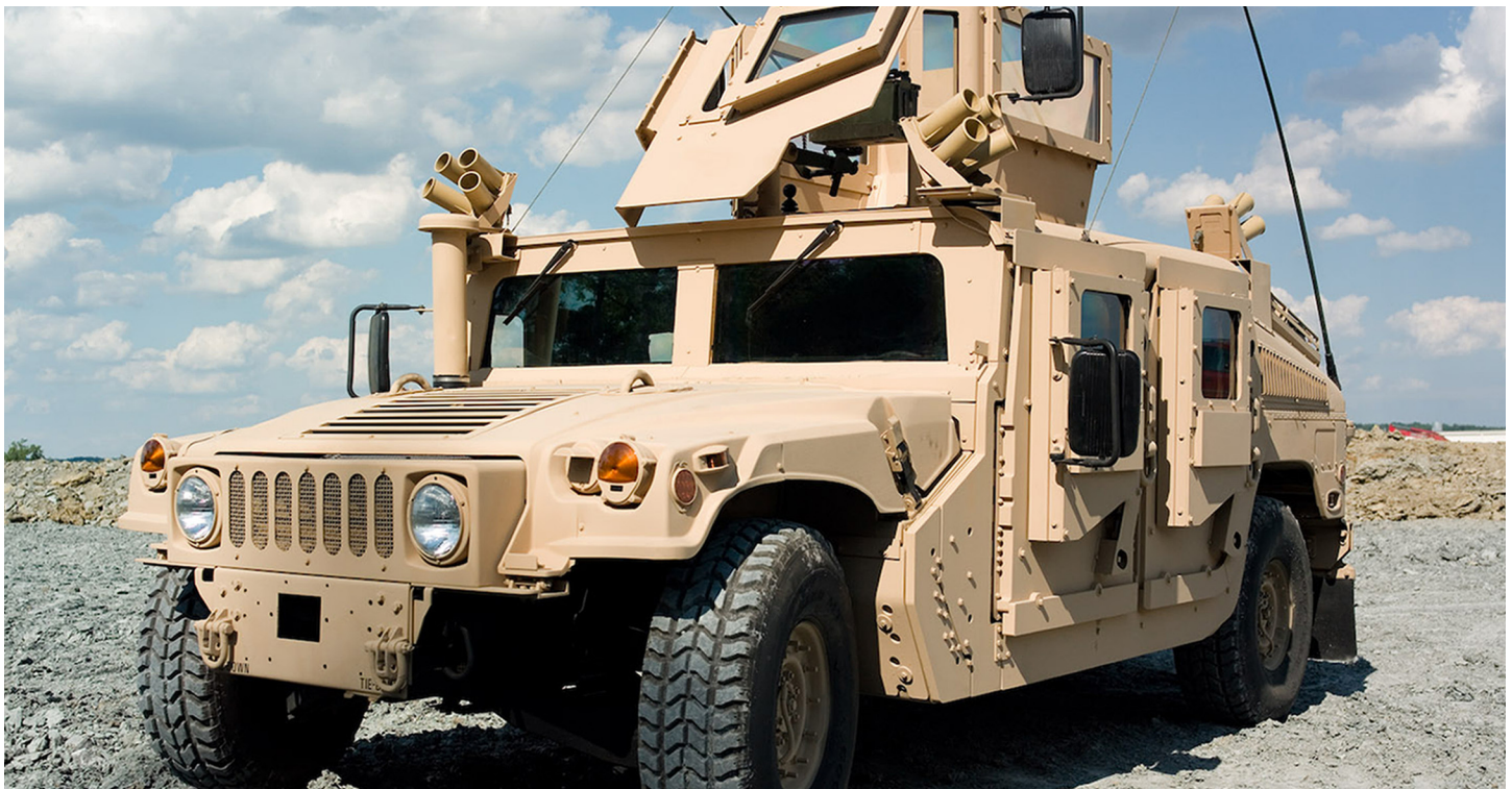
Up armored High Mobility Multipurpose Wheeled Vehicle (HMMWV)
