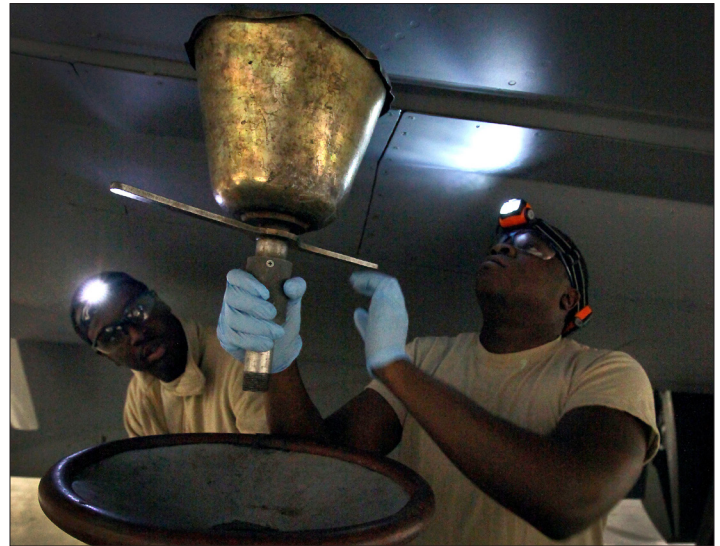
Staff Sgt. Delonte A. Williams, left, adjusts a funnel as Senior Airman Herbert L. Grant, both aircraft fuel systems journeymen, uses a cowbell to undo a screw prior to draining a fuel bladder.
