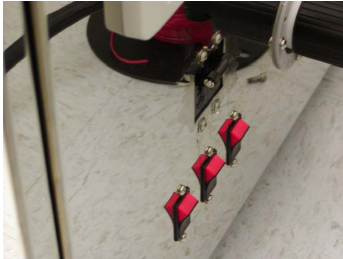
Four jumpers in the ON position on the rear panel of NX-2000 nanoimprinter
