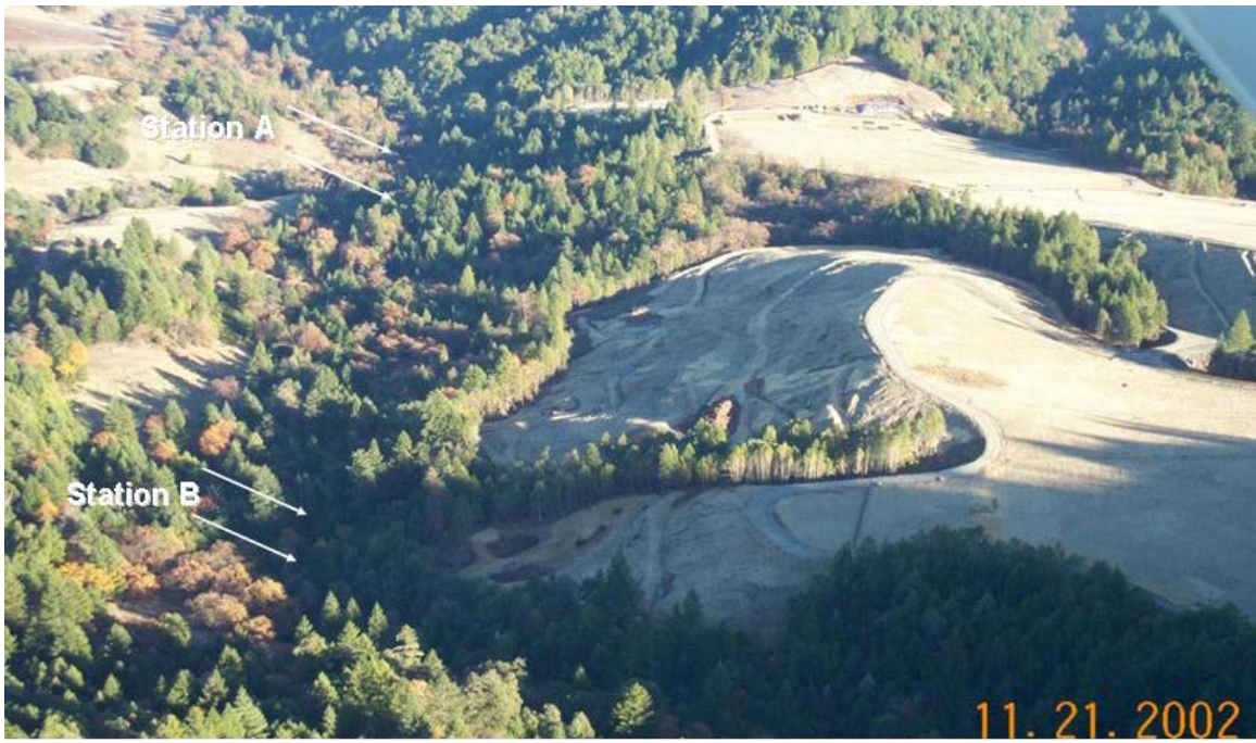
Figure 8. Aerial view of SF Mud Springs Creek and the barren land of the south cultivation unit at the onset of winter storms in 2002. Stream flow is from west, upstream (Station B in foreground) to east, downstream (Station A in background). Arrows indicate approximate location of the upstream and downstream turbidity sensors at each Station.
