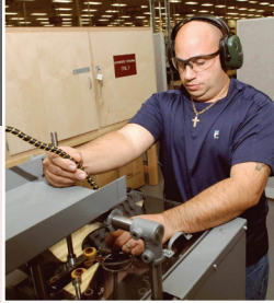
{ Photos, left to right: Robert Tambasco , an electronics mechanic at Tobyhanna Army Depot, guides a taped bundle of wire through a braiding machine. (U.S. Army photo by Tony Medici) • Charlene Nicholson , an electronics technician at Tobyhanna Army Depot, uses a Cirris table top cable tester to test a cable used in various Blue Force Tracking Kits. (U.S. Army photo by Steve Grzezdinski) }
