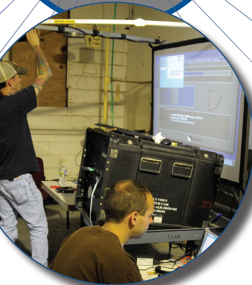
{ Electronics Technician Gerald Gaglio , left, and Electronics Worker Stephen Froncek test an AN/TSQ-243 Command Center System and Large Screen Display System while deployed to Fort Indiantown Gap. The systems are used to display visual battlefield information for commanders in the field. (Photos by Matt Jones) }
