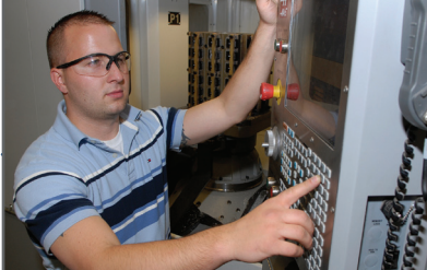
{ Left & Right: Night Vision Goggles, Center: Joshua Tedesco , a machine tool operator at Tobyhanna Army Depot, prepares the HAAS Horizontal Machining Center to do a pallet change while modifying helmet brackets to support enhanced hardware. Depot technicians are producing thousands of helmet brackets, which are used to mount night vision devices. – U.S. Army photo by Steve Grzezdziński }
