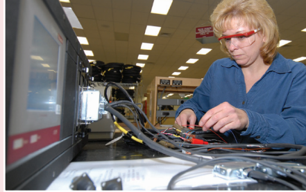
{ Photos, left to right: Robert Tambasco , an electronics mechanic at Tobyhanna Army Depot, guides a taped bundle of wire through a braiding machine. (U.S. Army photo by Tony Medici) • Charlene Nicholson , an electronics technician at Tobyhanna Army Depot, uses a Cirris table top cable tester to test a cable used in various Blue Force Tracking Kits. (U.S. Army photo by Steve Grzezdinski) }
