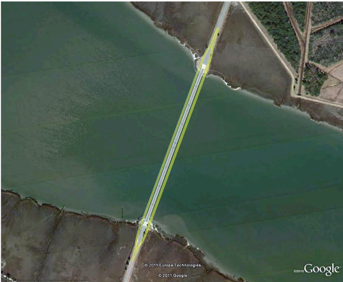
Figure 7. The new one lane bridge alignments are shown on an aerial photograph.
