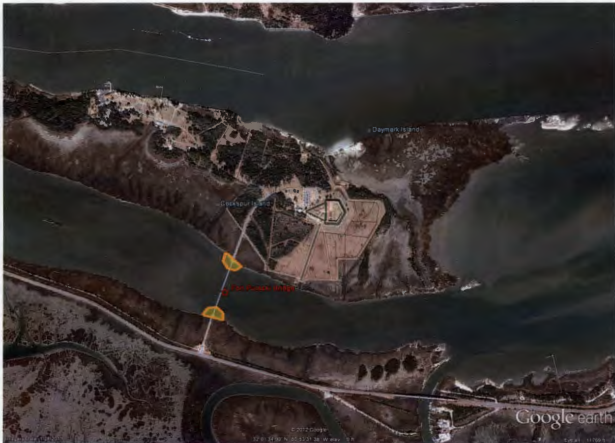
Figure 2. The 47-m behavioral impact zone for Atlantic sturgeon from the vibratory piling of sheet piles to create coffer dams around the two bridge abutments.
