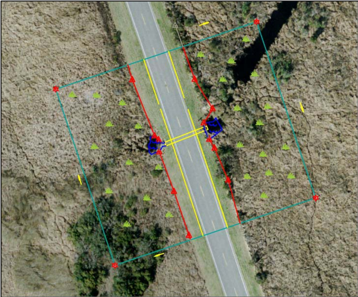
Figure 14. Delineated wetlands are shown surrounding the culvert at mile 3.13.
