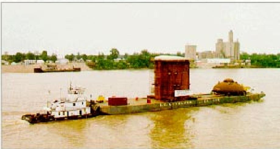
The vessel, head, internal items, and transport equipment, weighing a total of 2,200 tons, were loaded onto a 276-foot barge and shipped 750 miles up the Ohio River. After departing Mt. Vernon (bottom), the loaded barge passed under 49 bridges, including those at Cincinnati (top).
