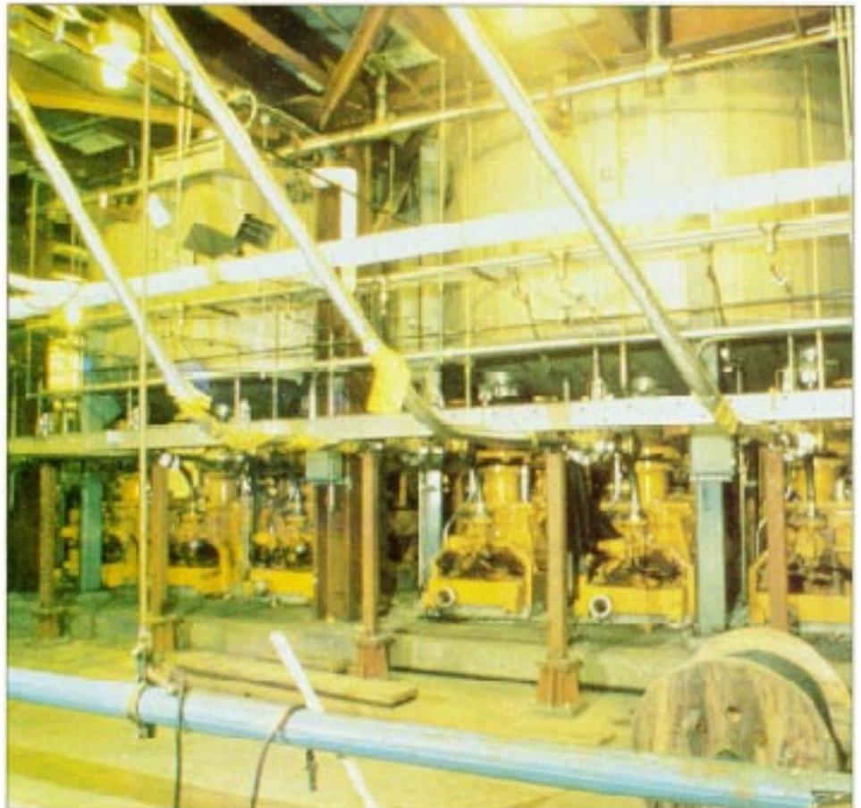
The fuel is pumped as a coal-water paste which is 25% water. A specific distribution of coal size is used to eliminate inter-particle motion and to make pumping the paste easier. The coal's moisture is measured on the weigh feeder and water is added to the mixer to prepare the paste. It then goes directly into a fuel feed hopper which has a 1-hour storage capacity.
