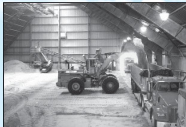
The gypsum cake is loaded onto trucks for delivery to the purchaser.
