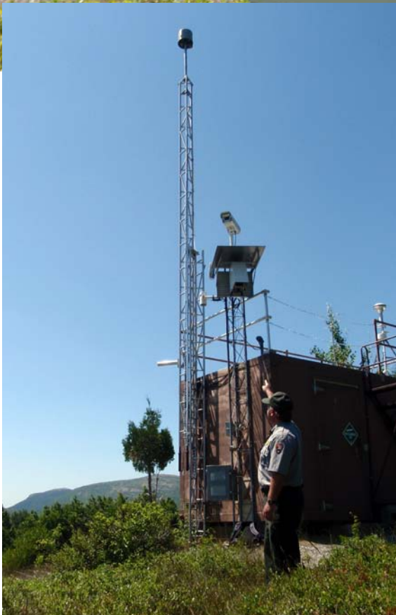
Air quality monitoring at Acadia National Park in Maine includes monitoring of mercury wet deposition (equipment pictured above) as well as visibility, ozone, and dry deposition of nitrogen and sulfur (equipment pictured to the left).
