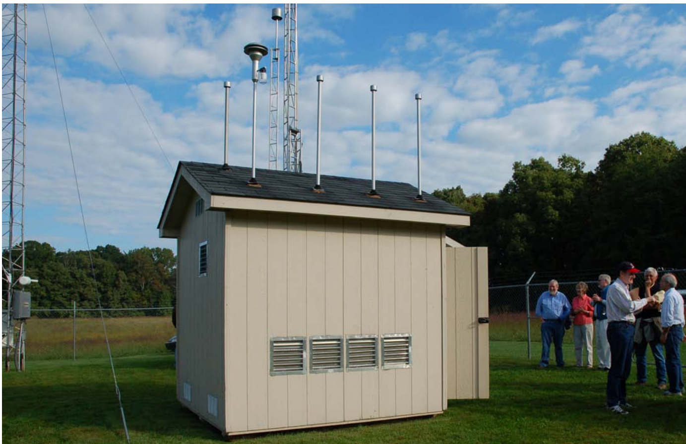
The IMPROVE (Interagency Monitoring of Protected Visual Environments) program monitors visibility conditions in National Parks and Wilderness Areas. IMPROVE monitoring stations, like the Houchin's Meadow station at Mammoth Cave National Park, Kentucky, use modular aerosol samplers to measure fine and total aerosol mass by pulling air through specialized filters which are routinely collected and analyzed.
