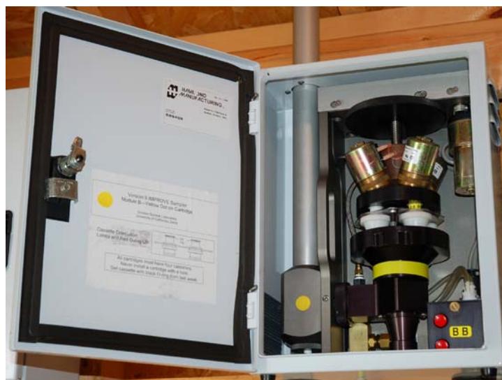
Top photo: The Houchin's Meadow IMPROVE monitoring station at Mammoth Cave National Park, Kentucky. Left: Inside the IMPROVE station. Below: Close-up of module B filter packs used to sample atmospheric PM 2.5, sulfate, and nitrate. Credit: National Park Service.
