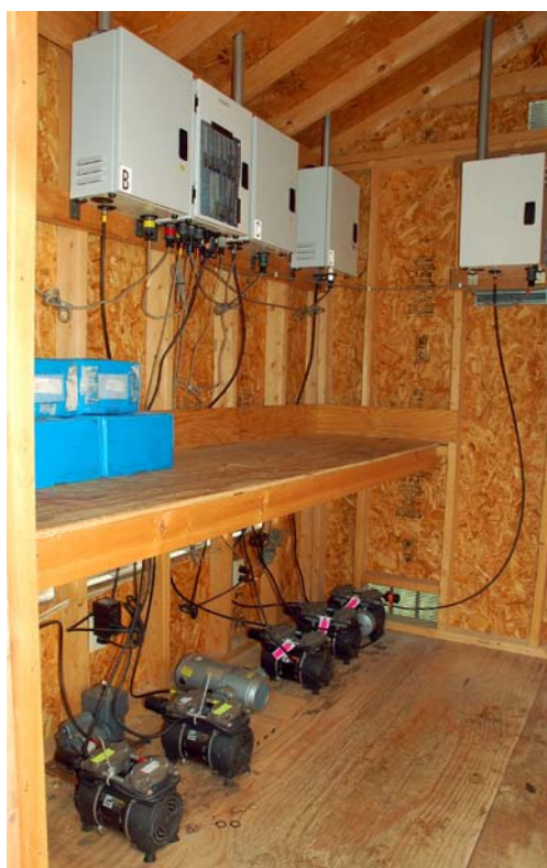
The IMPROVE (Interagency Monitoring of Protected Visual Environments) program monitors visibility conditions in National Parks and Wilderness Areas. IMPROVE monitoring stations, like the Houchin's Meadow station at Mammoth Cave National Park, Kentucky, use modular aerosol samplers to measure fine and total aerosol mass by pulling air through specialized filters which are routinely collected and analyzed.
