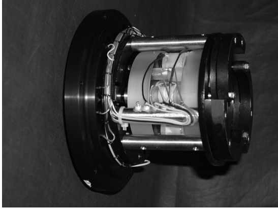
Fig. 1. Internal view of the MSFC/Hovermere CIV scanning FPI which incorporates (Cascade Optical Corporation) VUV coating technology with a resolving power of 22,100. This could be used as one element for the high resolution interferometer for a multiple Fabry-Perot etalon spectral filter for CIV described in the text. The interferometer length is 150 mm.
