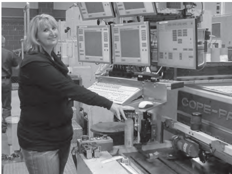
Cindy Rawlinson, Currency Overprinting Assistant Foreman, prepares press for printing of seals and serial numbers.
