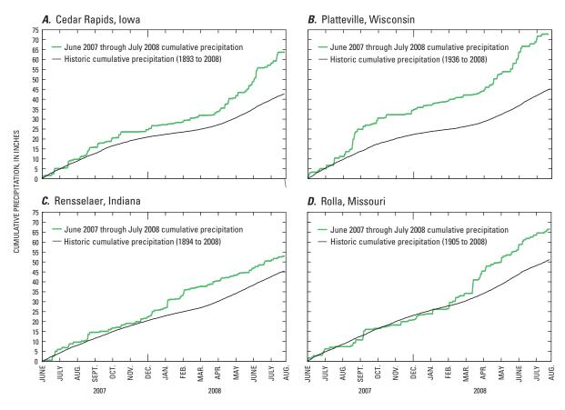
**Figure 6.** Cumulative precipitation totals from June 1, 2007, to July 31, 2008, in relation to historic average cumulative precipitation for selected sites in the Midwest. (National Climatic Data Center, 2008).
