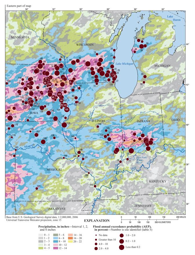
**Figure 12.** Cumulative precipitation totals for May 21 through June 14, 2008, and locations of U.S. Geological Survey streamgages in several Midwestern States with peak streamflows that had an annual exceedance probability less than 10 percent.—Continued
