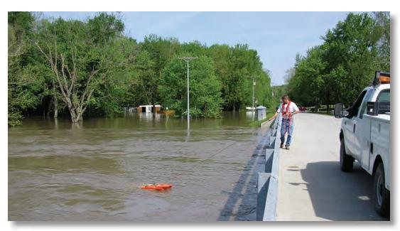
**Figure 2.** U.S. Geological Survey hydrographer measuring streamflow on the Platte River near Sharps Station, Missouri (USGS streamgage 06821190), with an acoustic Doppler current profiler (ADCP) mounted to a tethered boat to collect velocity and depth readings that are sent by radio link to a laptop computer inside the field vehicle. The gage house for this site can be seen in the background. Photograph by Chris Rowden, USGS.
