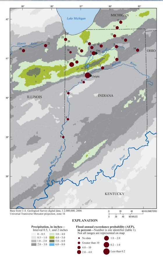
**Figure 7.** Cumulative precipitation totals for January 7–9, 2008, and locations of U.S. Geological Survey streamgages in Illinois, Indiana, and Michigan with peak streamflows that had an annual exceedance probability less than 10 percent.
