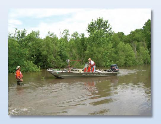
USGS hydrographers preparing to make a boat measurement of the streamflow coming across the road on the Cedar River near Conesville, Iowa (USGS streamgage 05465000). Photograph by Scott Strader, USGS.
