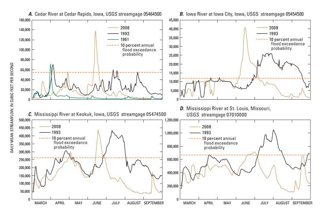
**Figure 18.** Streamflow for selected U.S. Geological Survey streamgages for the 2008 flood period and previous major floods, and the 10-percent annual exceedance probability for each site.
