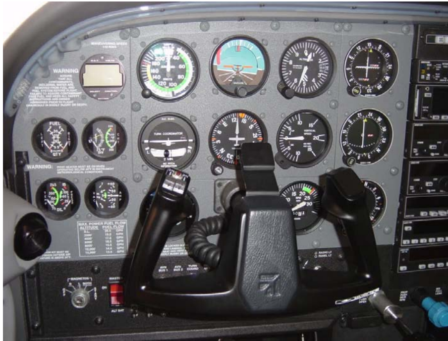
Figure 1. Example of a light aircraft conventional cockpit.
