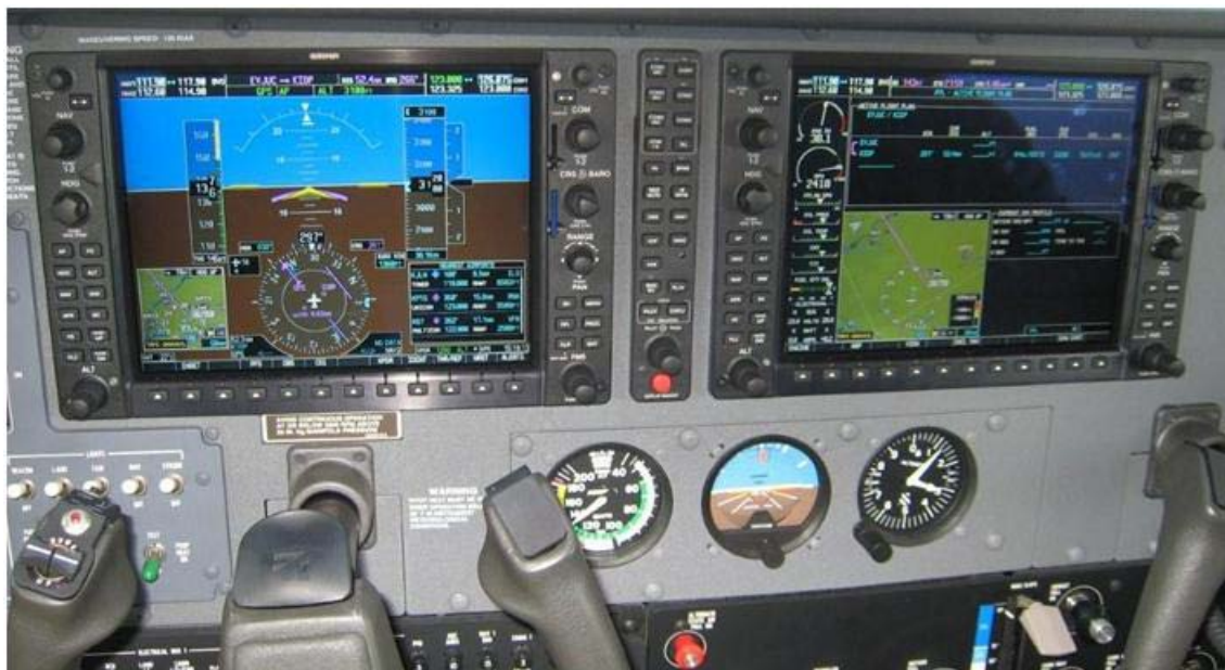
Figure 2. Example of a light aircraft glass cockpit.
