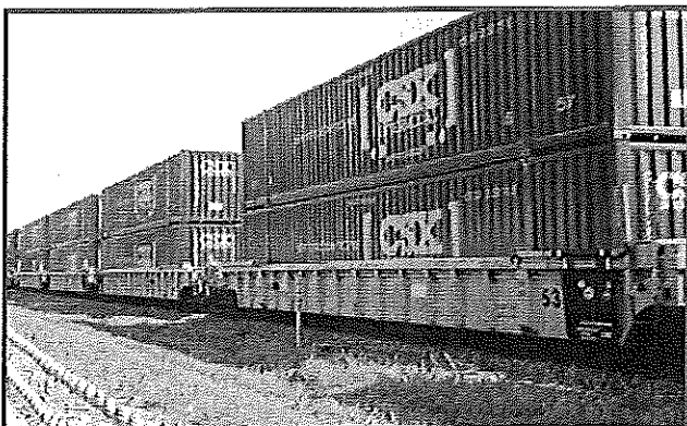
Modifying clearances for double-stack containers will improve the flow and efficiency of freight by expanding capacity.
