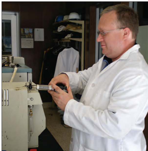
Figure 4-4. Lab Personnel Using Syringe to Inject GC.
