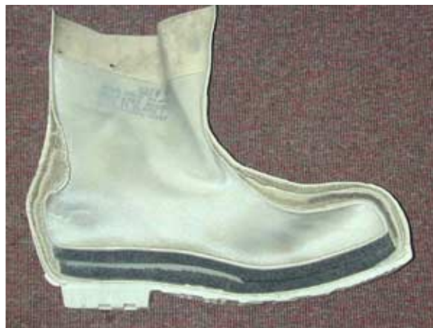
Fig. 18-1. The vapor barrier (VB) boot is standard issue for military personnel assigned or deployed to arctic environments. Often nicknamed the "Mickey Mouse" boot, it provides excellent protection from cold under most conditions down to -50^{\circ}\text{F} . Air trapped between two layers of rubber and a thick felt sole pad provide the insulation. A release valve (not shown) is present to relieve pressure when traveling in unpressurized aircraft. VB boots should be inspected at least annually to ensure that the trapped air layer is tightly sealed. Photograph: Courtesy of US Army Northern Warfare Training Center, Fort Greeley, Alaska.
