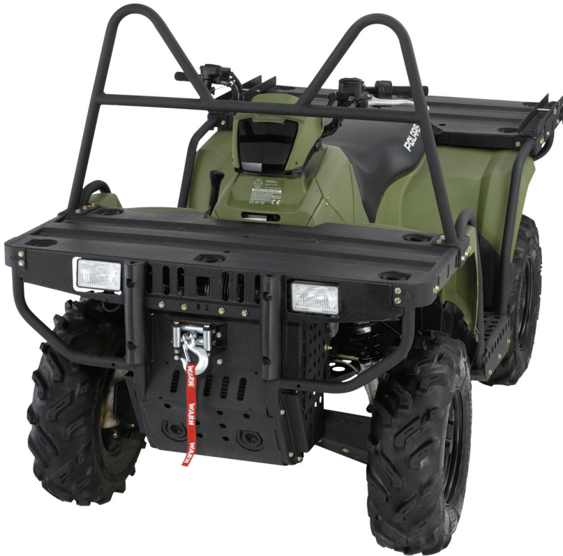
Figure 14. Polaris Sportsman military vehicle. It is a four-wheel, all-terrain vehicle that can carry one person and a load up to 204 kg. Photograph: Courtesy of Justin Burke, Marketing Manager, Polaris Defense, Medina, Minn. From http://www.polarisindustries.com .
