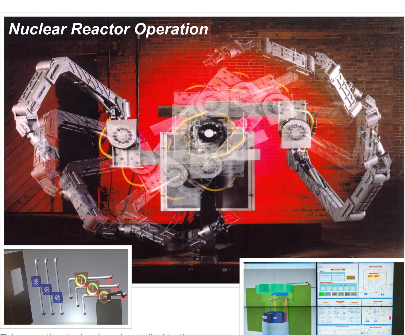
Teleoperation technology is applied to the operation and maintenance of nuclear reactors and remotely-located energy facilities, such as ocean-based oil rigs and wind mills. Advanced man-machine interface and interactive simulation allows hands-on experience and training of such operation.
