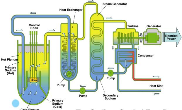
The Sodium Cooled Fast Reactor (SFR) enables multirecycle of actinides to avoid nuclear waste accumulation and improve uranium utilization; its main missions are consumption of actinides recovered from discharged light water reactor (LWR) fuel and generation of electricity.
