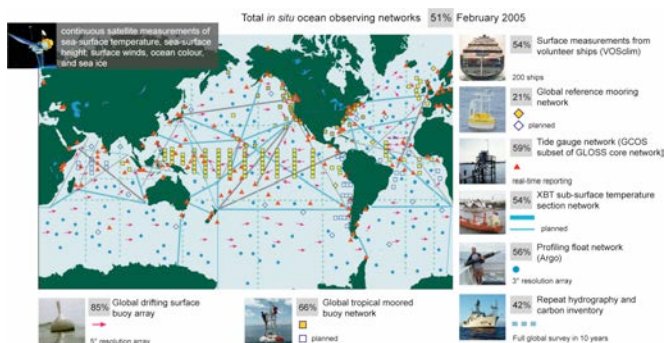
Figure 2: A schematic of the initial composite ocean observing system, including the current status against the targets of JCOMM and the GCOS Implementation Plan (GCOS-92), maintained by the international GOOS Project Office. The statistics were calculated by OCO as a national contribution to the international effort. This report was issued in February as the system passed the 50% mark.
