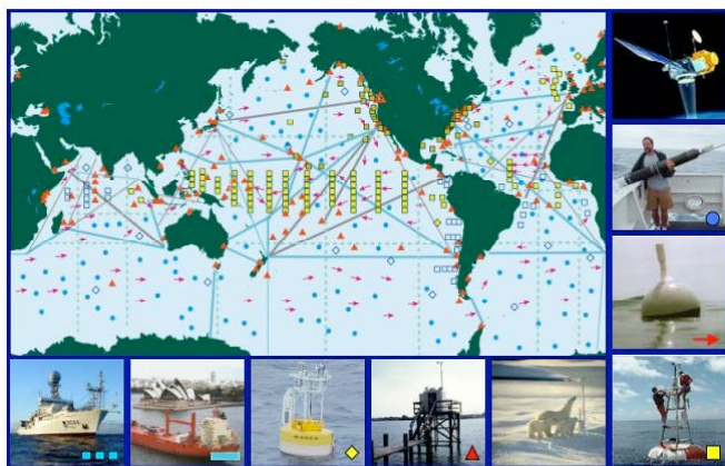
Figure 1. The Networks that make up the Sustained Ocean Observing System for Climate are (from lower left to upper right): Dedicated Ships, Ships of Opportunity, Ocean Reference Stations, Tide Gauge Stations, Arctic Observing Systems, Tropical Moored Buoys, Surface Drifting Buoys, Argo Profiling Floats, and Continuous Satellite Missions for sea surface temperature, sea surface height, surface vector winds, ocean color, and sea ice. Not illustrated are the Data & Assimilation Subsystems and Product Delivery.
