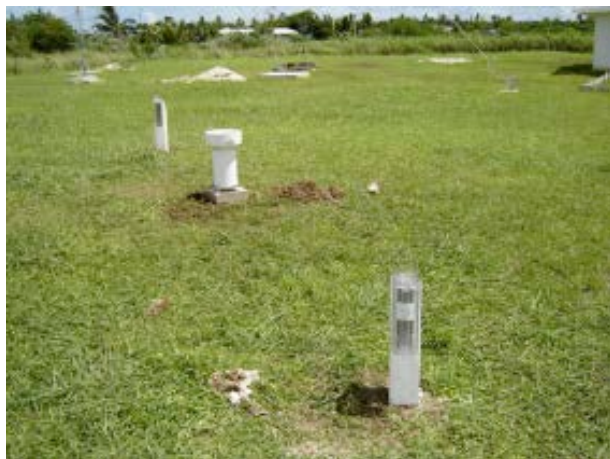
Figure 4. Pilot Project Testbed setup in Niue. The METONE tipping bucket gauge can be seen in between the two manual raingauges
