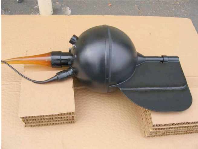
Figure 1. Photograph of the surface float of a SVP-W wind drifter that is attached to a thermistor chain, to form an ADOS drifter. The wind speed is determined from ambient noise with a hydrophone whose cable is protruding at an angle from the bottom of the float and the wind direction is determined from conditionally sampling the vane.
