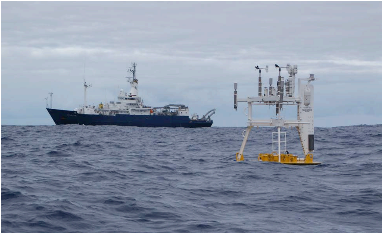
Figure II-2: The Stratus buoy with RV Melville in the background, taken during comparison of ship meteorological sensors (mounted on the tower on the bow) and buoy sensors.
