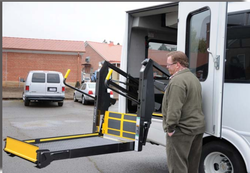
The Wheelchair lift is demonstrated during the delivery of the buses
